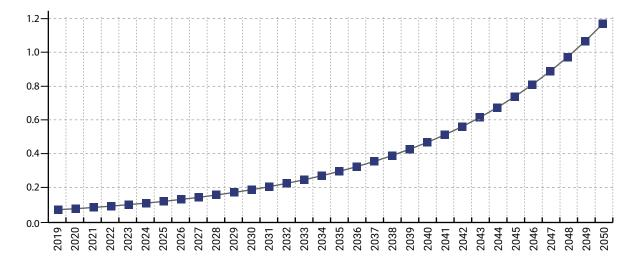
Figure 17 Evolution scenario of photovoltaic installed capacity in Mato Grosso's residential sector on the horizon 2050. Unit: GWpeak.
